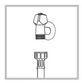
1. Connect the supply pipe by screwing it to a cold water tap using a ¾ gas threaded connection (see figure).
